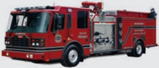
INUNDATOR SUPER PUMPER 38,000+ LPM from pressurized source 20,000+ LPM from draft
