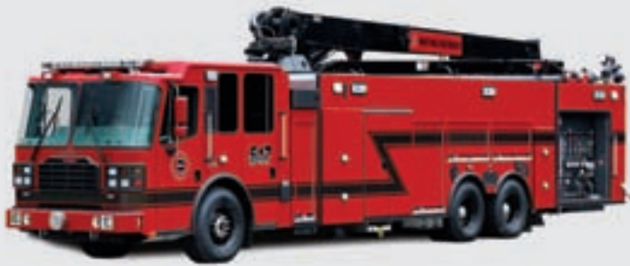
INUNDATOR SP-85 BOOM 15,000+ LPM from aerial discharge 15,000+ LPM from dual rear monitors
